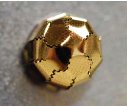
Close up of hexagonally-shaped pixels from the origami sensor draped over a dome shape, with perfectly jointing seams. Yei Hwan Jung and Kan Zhang.
