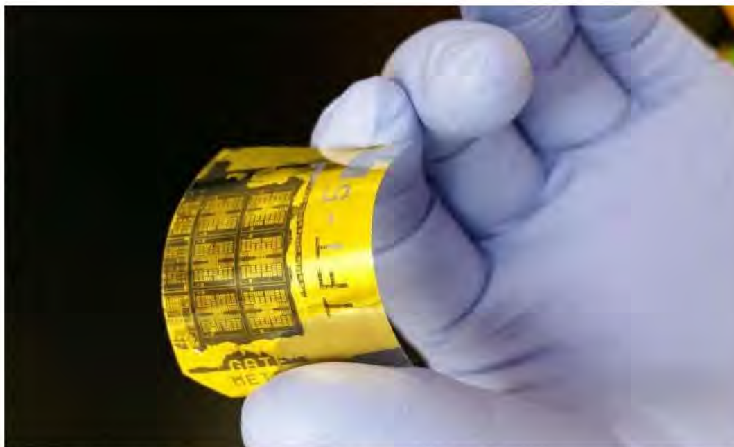
Developed by UW-Madison electrical engineers, this unique phototransistor is flexible, yet faster and more responsive than any similar phototransistor in the world. Credit: Jung-Hun Seo
